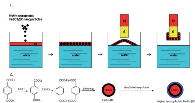
Fig. 7 Illustration of (1) oil removal from the water surface and (2) the preparation of the NPs. Reprinted with permission.<sup>113</sup> Copyright 2010 American Chemical Society.
