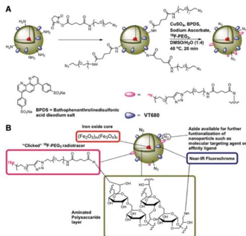
Fig. 5 Preparation of <sup>18</sup>F-CLIO; (A) derivatisation of primary amines followed by chemoselective "click" of the <sup>18</sup>F-PEG radiotracer; (B) schematic of <sup>18</sup>F-CLIO. Reprinted with permission.<sup>96</sup> Copyright 2009 American Chemical Society.
