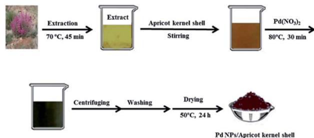
Fig. 6 Synthesis procedure of Pd NPs/Apricot kernel shell. Reprinted with permission from Elsevier. 108
