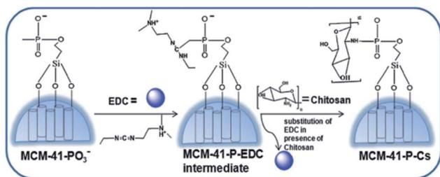
Fig. 3 Schematic procedure of the preparation of chitosan coated mesoporous silica NPs. Reprinted with permission from The Royal Society of Chemistry.<sup>71</sup>
