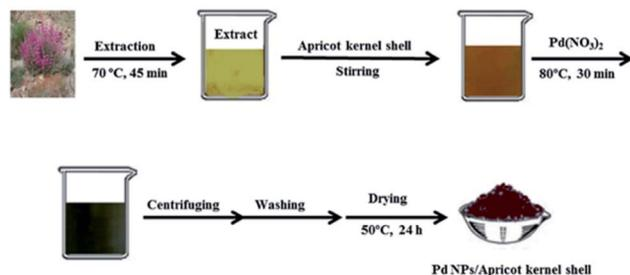
Fig. 6 Synthesis procedure of Pd NPs/Apricot kernel shell. Reprinted with permission from Elsevier.<sup>108</sup>
