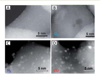
Fig. 2 (A) HAADF-STEM images of the as-prepared 1.66 wt% Pt $_1$ / Fe $_2$ O $_3$  SAC and the samples treated in (B) O $_2$ , (C) H $_2$ , and (D) CO at 250 °C for 2 h. Reproduced with permission. <sup>50</sup> Copyright 2018, IOP Publishing Ltd.
