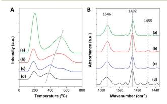
Fig. 4 (A) NH<sub>3</sub>-TPD profiles and (B) FTIR spectra obtained after the desorption of pyridine at 150 °C of (a) mordenite, (b) MOR@ZSM-5(SS), (c) MOR@ZSM-5(CS), and (d) ZSM-5-NS.
