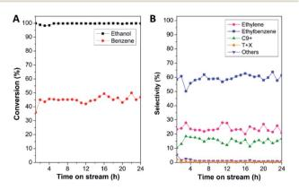
Fig. 5 (A) Reaction conversion (%) and (B) product selectivity (%) over the MOR@ZSM-5(CS) sample in benzene alkylation at 450  $^{\circ}$ C as a function of time on stream (TOS) for 24 h.
