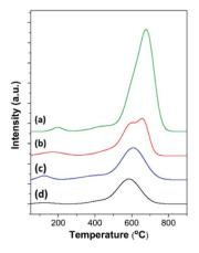
Fig. 7  $O_2$ -TPO profiles of the spent catalysts: (a) mordenite, (b) MOR@ZSM-5(SS), (c) MOR@ZSM-5(CS), and (d) ZSM-5-NS taken after the catalytic test for the alkylation of benzene with ethanol at 450 °C for 24 h.
