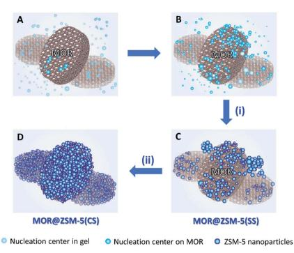
Scheme 1 Illustration of the proposed formation pathways of MOR@ZSM-5(SS) and MOR@ZSM-5(CS) via (i) single-step crystallization (via A, B, and C); (ii) continuous crystallization of nanocrystalline ZSM-5 on the mordenite surfaces (D).
