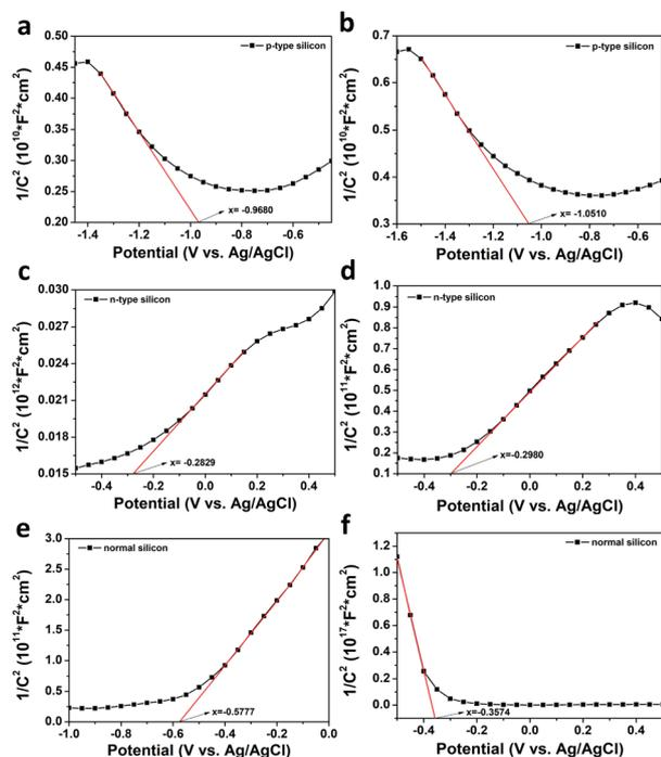
Fig. 6 Mott–Schottky test results on different substrates.
