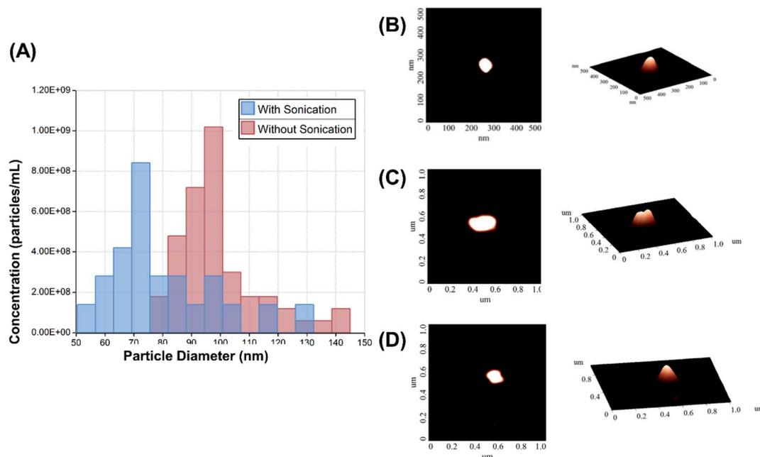
**Fig. 3** (A) The size distribution of the echogenic exosomes as measured by the qNano (with and without sonication). Atomic force microscopy images (B–D) of echogenic exosomes. These exosomes range between 60 to 90 nm in diameter after they undergo the protocol to make them echogenic.
