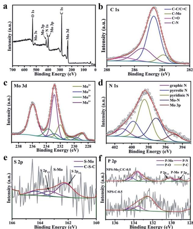
Fig. 3 (a) XPS survey spectra of NPS-Mo<sub>2</sub>C/C-0.5 and the corresponding high-resolution spectra of (b) C 1s, (c) Mo 3d, (d) N 1s, and (e) S 2p. (f) High-resolution spectra of NPS-Mo<sub>2</sub>C/C-0.5 and NPS-C-0.5.
