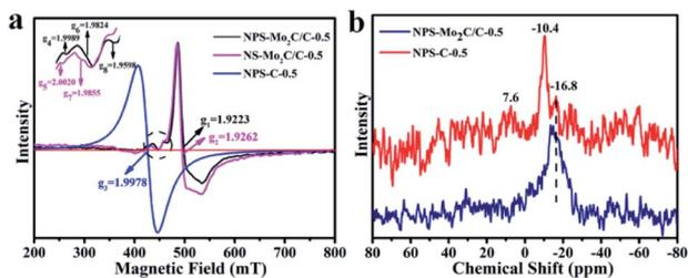
Fig. 4 (a) Room temperature EPR spectra of NPS-Mo<sub>2</sub>C/C-0.5, NS-Mo<sub>2</sub>C/C-0.5 and NPS-C-0.5. (b) <sup>31</sup>P solid-state MAS NMR spectra of NPS-Mo<sub>2</sub>C/C-0.5 and NS-Mo<sub>2</sub>C/C-0.5.
