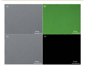
Fig. 5 Reflected bright-field (A) and fluorescence microscopy images (B) for the fluorous porous silicon particles deposited on a silicon wafer after treatment with FITC-C $_8$ F $_{15}$ . Reflected bright-field (C) and fluorescence microscopy images (D) for the unmodified porous silicon particles deposited on a silicon wafer after treatment with FITC-C $_8$ F $_{15}$ .
