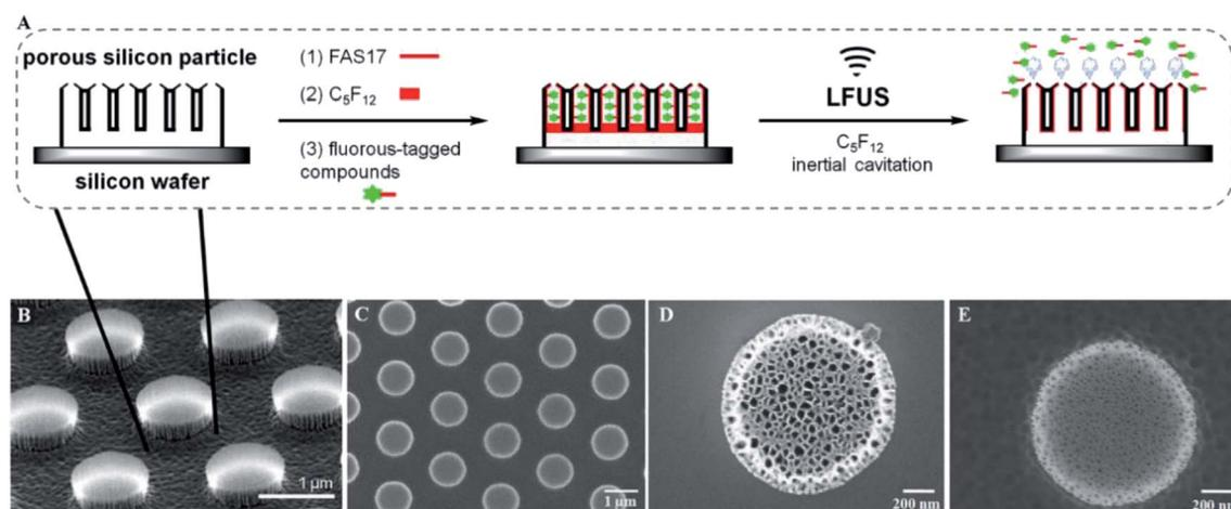
Fig. 1 (A) Schematic illustration of the general procedure for the low frequency ultrasound triggered release of fluororous-tagged compounds. The tilted view (B) and top view (C) of the SEM images of the discoidal porous silicon particles deposited on a silicon wafer. SEM images of the porous morphology of the release layer (D) and the device layer (E).
