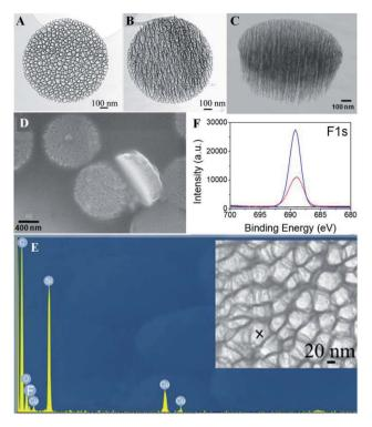
Fig. 2 TEM images of the release layer (A) and device layer (B), and tilt view (C) and SEM image (D) of the fluorous discoidal porous silicon particles. (E) EDS spectrum of the area marked with an "X" on the fluorous porous silicon particles. (F) High-resolution F1s scans of the unmodified porous silicon particles (black line), fluorous porous silicon particles (red line), and FITC- $C_8F_{15}$  incorporated fluorous porous silicon particles (blue line).
