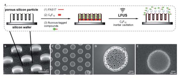
Fig. 1 (A) Schematic illustration of the general procedure for the low frequency ultrasound triggered release of fluorous-tagged compounds. The tilted view (B) and top view (C) of the SEM images of the discoidal porous silicon particles deposited on a silicon wafer. SEM images of the porous morphology of the release layer (D) and the device layer (E).
