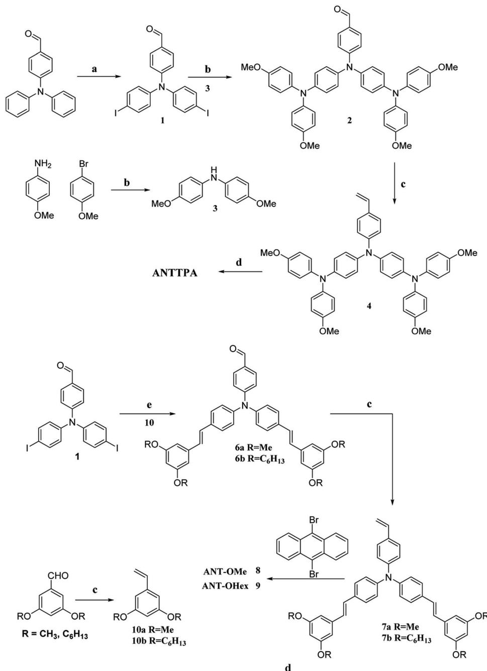
**Scheme 1** Synthetic route of the designed HTMs ANTPA, AOME, and AOHE. Reagent and conditions: (a)  $\text{KIO}_3/\text{KI}$ ,  $\text{CH}_3\text{COOH}$ ,  $80^\circ\text{C}$ ; (b) bis(*tert*-*tert*-butylphosphine)palladium(0),  $\text{NaOtBu}$ , toluene,  $95^\circ\text{C}$ , overnight; (c) methyltriphenylphosphonium iodide, DCM,  $\text{KOtBu}$ , RT; (d and e)  $\text{Pd}(\text{OAc})_2$ , tetrabutylammonium bromide, triethylamine, DMF/toluene (1 : 1),  $95^\circ\text{C}$ .
