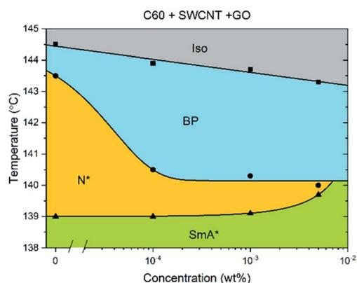
Fig. 6 Phase diagram of CE8 with C60, GO and SWCNT all added together in a 1 : 1 : 1 ratio. The concentration is expressed as the total nanoparticle content by weight %. The uncertainty of the temperature measurements is of the order of the data points,  $\sim 0.1$  K. The solid lines are a guide to the eye.
