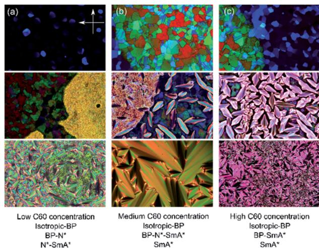
Fig. 3 Illustrative POM textures showing the effect of (a) low, (b) medium, and (c) high fullerene concentration and temperature (vertical) on the phase behavior of CE8. The BP–N\*–SmA\* triple point texture can be seen in the central texture micrograph. The orientations of the polarizer and analyzer are the same in all the images.
