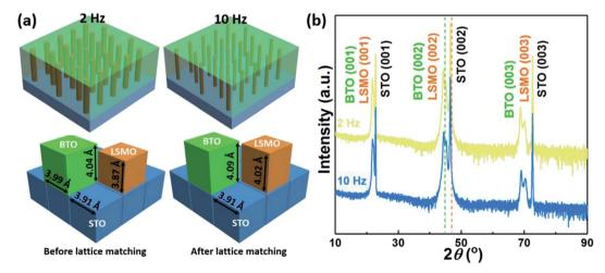
Fig. 1 (a) Designed 3D schematic drawing of the: BTO: LSMO VAN thin films deposited at 2 Hz and 10 Hz (top); lattice parameters of BTO, LSMO and STO before and after the matching (bottom). (b)  $\theta$ –2 $\theta$  XRD scans of BTO: LSMO thin films deposited at 2 Hz and 10 Hz. The green and orange dashed lines indicate the (002) peak positions of the bulk BTO and LSMO, respectively.
