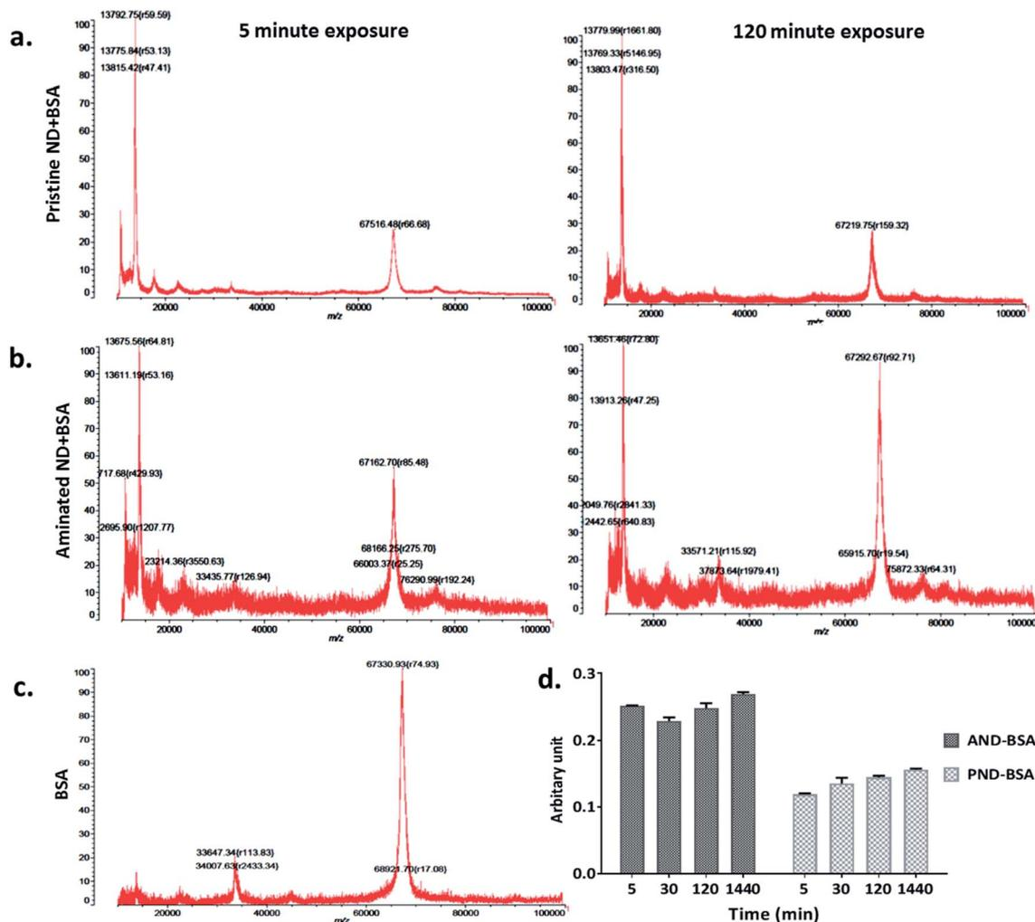
**Fig. 3** Time resolved measurements of BSA corona formation: (a) MALDI-TOF spectra of pristine nanodiamonds exposed to BSA for 5 min and 120 min. (b) MALDI-TOF spectra of aminated nanodiamonds exposed to BSA for 5 min and 120 min. (c) Spectrum of the BSA standard; (d) micro BCA assay results of aminated and pristine nanodiamonds exposed to BSA.
