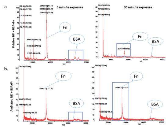
Fig. 5 Time-resolved changes in the amount of protein on the nanodiamonds exposed to an equal mixture of BSA and FN9-10 for 5 and 30 min – MALDI-TOF: (a) pristine nanodiamonds and (b) aminated nanodiamonds.
