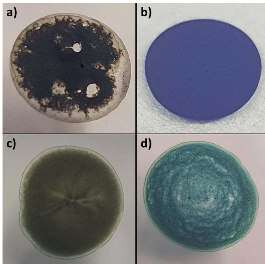
Fig. 7 Photographs of dropcast films on ITO of (a) H<sub>2</sub>mim<sup>+</sup>TCNQ<sup>-</sup>, (b) Zn<sup>2+</sup>(TCNQ<sup>-</sup>)<sub>2</sub>(H<sub>2</sub>O)<sub>2</sub>, and PSI-Zn-H<sub>2</sub>mim-TCNQ both (c) before and (d) after electrochemical cycling in 100 mM Zn(OAc)<sub>2</sub>.
