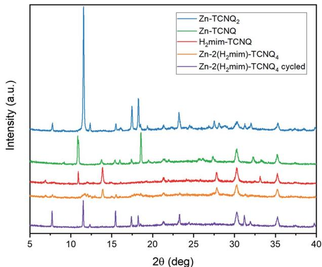
Fig. 9 X-ray diffraction patterns of TCNQ complexes without PSI, revealing the cation replacement of H<sub>2</sub>mim with Zn during electrochemical cycling.
