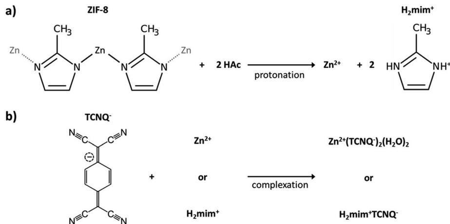
Fig. 1 Schematic of (a) the breakdown of ZIF-8 by acetic acid to release  $\text{Zn}^{2+}$  and  $\text{H}_2\text{mim}^+$  cations and (b) the subsequent reaction of these cations with  $\text{TCNQ}^-$  to form insoluble charge transfer complexes.
