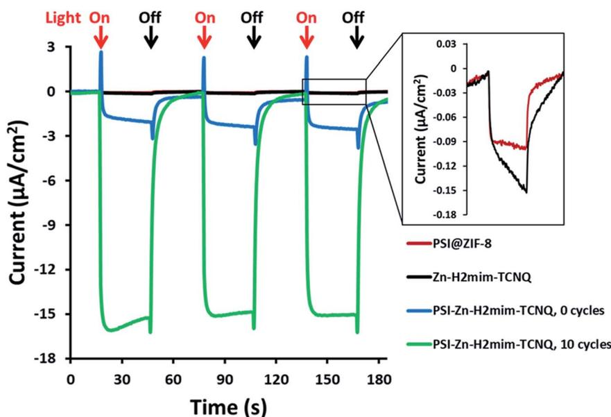
**Fig. 5** Photocurrent production of prepared samples in the presence of 4 mM methyl viologen as the electron scavenger and 100 mM Zn(OAc)<sub>2</sub>, illuminated by 300  $\text{W m}^{-2}$  red light in 30 second intervals. All measurements at OCV.
