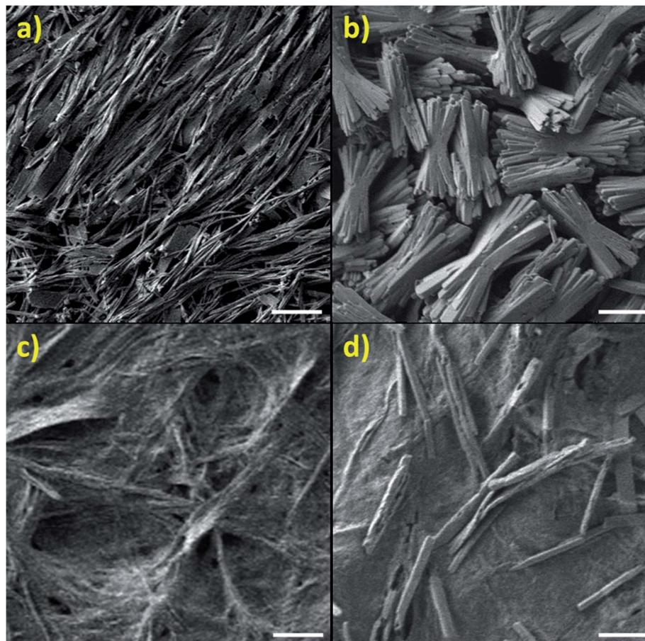
Fig. 8 SEM images of dropcast films on ITO of (a) H<sub>2</sub>mim<sup>+</sup>TCNQ<sup>-</sup>, (b) Zn<sup>2+</sup>(TCNQ<sup>-</sup>)<sub>2</sub>(H<sub>2</sub>O)<sub>2</sub>, and PSI-Zn-H<sub>2</sub>mim-TCNQ both (c) before and (d) after electrochemical cycling in 100 mM Zn(OAc)<sub>2</sub>. Scale bar 2 microns.
