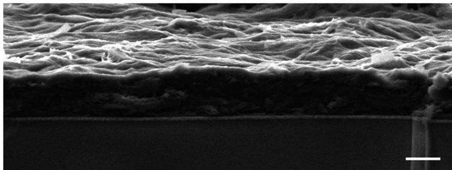
Fig. 2 Cross section of a PSI-Zn-H<sub>2</sub>mim-TCNQ film on ITO. Scale bar 2 microns.
