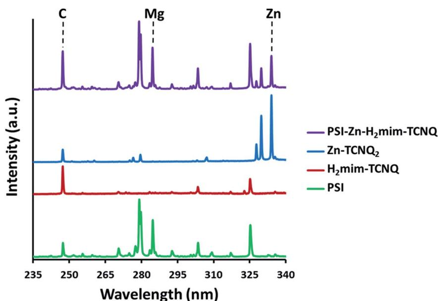
Fig. 4 Elemental emissions from laser-induced breakdown spectroscopy. The presence of Mg and Zn signatures confirms both intact chlorophyll and blended TCNQ salts.
