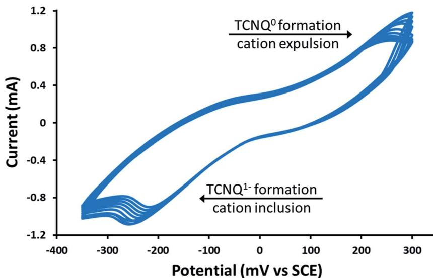
Fig. 6 Cyclic voltammety curves of a PSI-Zn-H<sub>2</sub>mim-TCNQ film in 100 mM Zn(OAc)<sub>2</sub>, scanned at 50 mV s<sup>-1</sup>.
