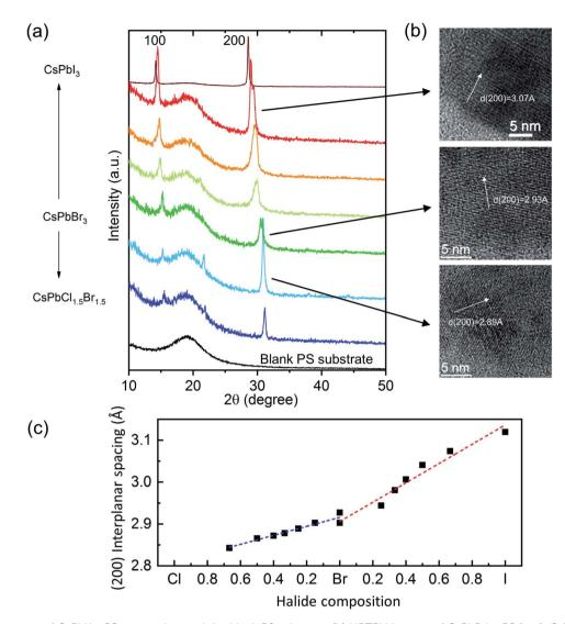
Fig. 2 (a) XRD patterns of CsPbX<sub>3</sub>-PS composites and the blank PS substrate. (b) HRTEM images of CsPbBrl<sub>2</sub>-PS (top), CsPbBr<sub>3</sub>-PS (middle), CsPbCl<sub>1.5</sub>Br<sub>1.5</sub>-PS (bottom) samples. (c) Interplanar spacings of (200) faces derived from XRD patterns of samples with different halide compositions
