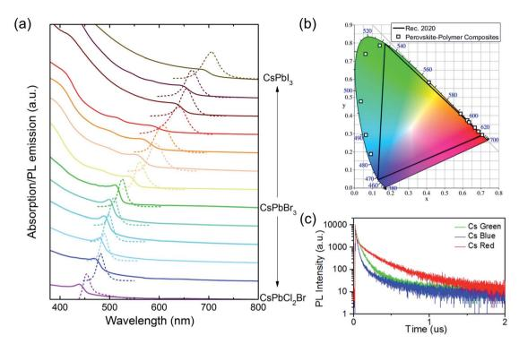
Fig. 3 Optical properties of  $CsPbX_3-PS$  composite films. (a) UV-vis absorption (solid lines) and PL emission (dashed lines) spectra. (b) Color coordinates of  $CsPbX_3-PS$  PL emission properties shown in the CIE 1931 color space. The Rec. 2020 (black line) color standard is shown for comparison. (c) PL decay curves of blue, green and red  $CsPbX_3-PS$  composite films under 375 nm excitation.
