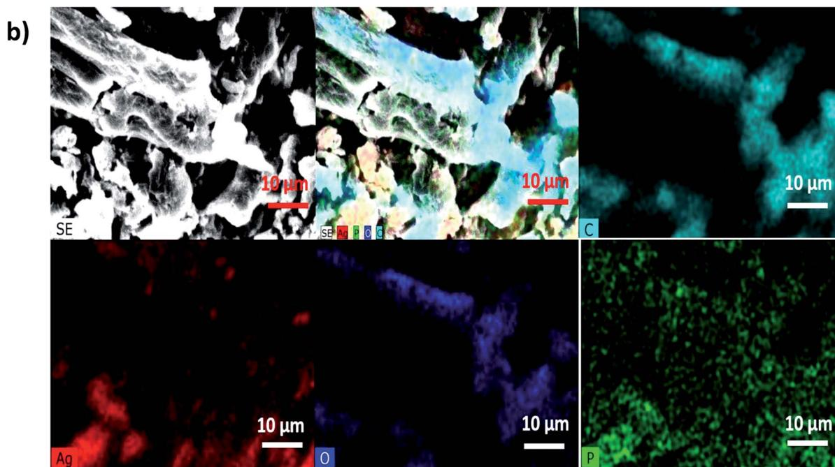
Fig. 1 (a) X-ray diffraction patterns of cellulose supported  $\text{Ag}_3\text{PO}_4$  nanostructures [Ag-0–Ag-8]. (b) SEM-EDX mapping images of cellulose supported silver phosphate nanostructures (Ag-8).
