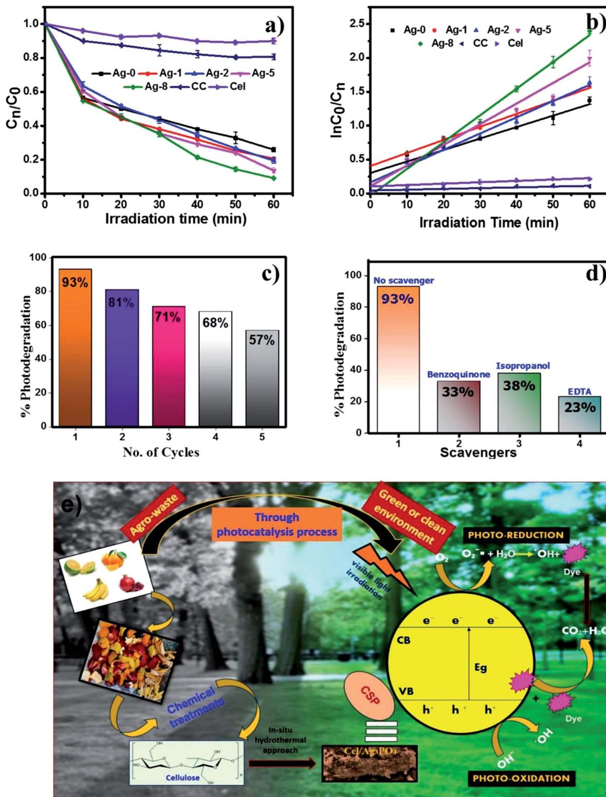
Fig. 6 (a and b) Comparative study of kinetic linear simulation of photo degradation of RhB dye using bare Ag<sub>3</sub>PO<sub>4</sub>, cellulose, commercial cellulose and cellulose supported nanostructures. (c) Recyclability tests of the Ag-8 photocatalyst. (d) Scavenger studies for Ag-8. (e) Proposed photodegradation pathway for Ag-8.
