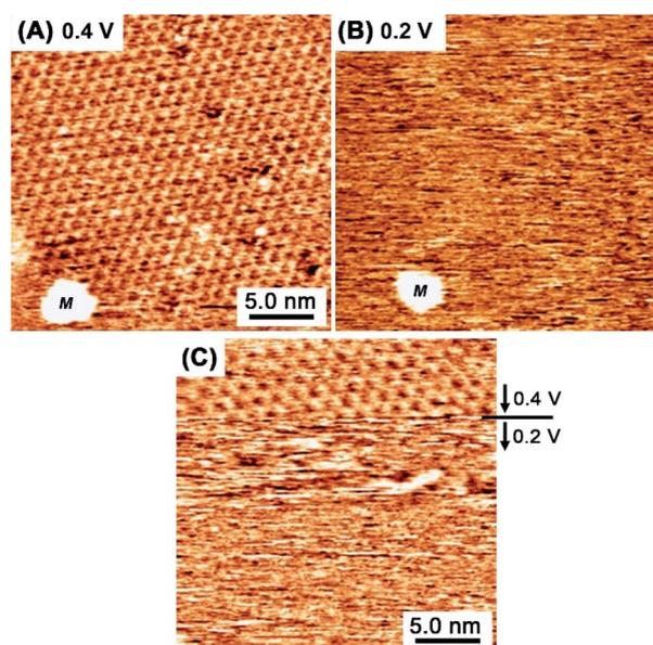
Fig. 4 *In situ* STM images obtained at 0.4 V (A) and 0.2 V (B) in a mixed aqueous solution comprising TAB and BTA. (A) and (B) were captured at the same location on the Au(111) surface, where “M” is an aggregated island used as a fiducial marker. During the scanning in (C), the potential was abruptly changed from 0.4 V to 0.2 V at the marked line.
