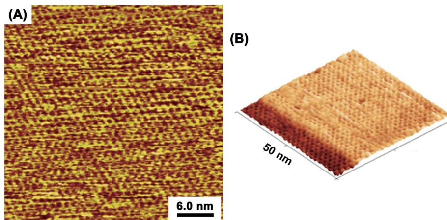
Fig. 1 *In situ* scanning tunneling microscopy (STM) images ((A) topographic image; (B) 3D image) of a TAB–BTA honeycomb network nanosheet on Au(111). The images were captured at open-circuit potential in a solution containing TAB and BTA. Honeycomb structures fabricated on upper and lower atomic terraces including Au single atomic steps are shown.
