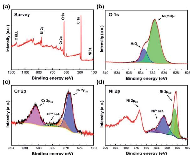
Fig. 4 XPS spectra of Ni<sub>2</sub>Cr<sub>1</sub>-LDNs: survey (a), and fitting spectra of O 1s (b), Cr 2p (c) and Ni 2p (d).
