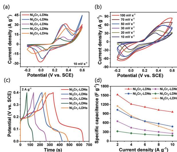
Fig. 5 (a) CV curves of LDN and LDH electrodes at a scan rate of 10 mV s<sup>-1</sup>, (b) CV curves of Ni<sub>2</sub>Cr<sub>1</sub>-LDNs at various scan rates from 5 to 100 mV s<sup>-1</sup>, (c) GCD curves of LDNs and LDHs at a current density of 2 A g<sup>-1</sup>, and (d) specific capacitances of LDN and LDH electrodes at different current densities.
