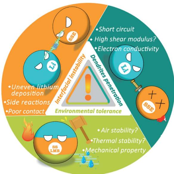
Fig. 1 Three potentially dangerous aspects of SSLMBs.
