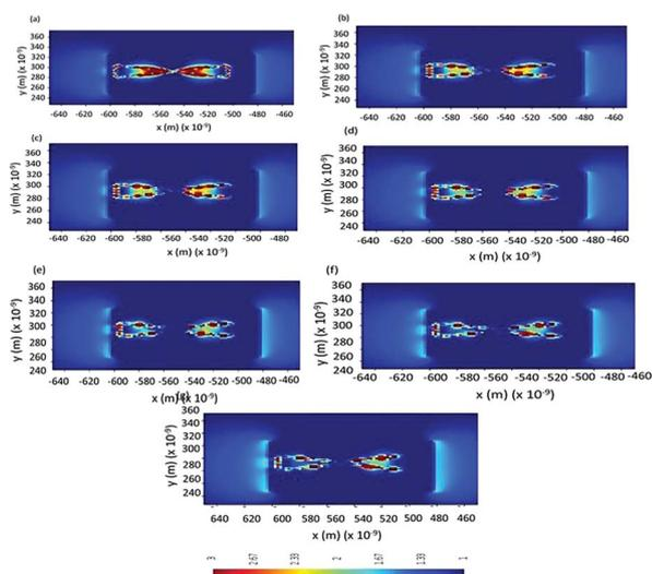
Fig. 6 FDTD simulations of electric field calculations between Au nano-urchin spikes distributed on amyloid beta fibrils with various refractive index values: (a) 1.6, (b) 1.65, (c) 1.7, (d) 1.75, (e) 1.8, (f) 1.85, and (g) 1.9, respectively (approximation for beta amyloid fibrillation).
