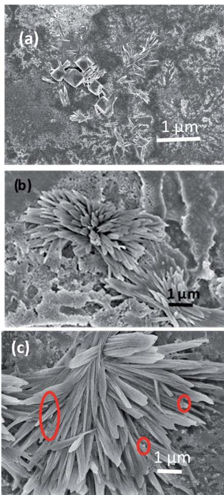
Fig. 8 FESEM images of  $A\beta_{1-42}$  mixed with Au nano-urchins for incubation times of 5 minutes (lag phase) (a), 40 minutes (growth phase) (b) and 90 minutes (steady phase) (c); red circles indicate Au nano-urchins attached to  $A\beta_{1-42}$  fibrils.
