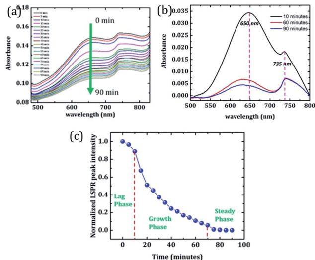
Fig. 5 (a) Absorbance vs. wavelength plots for the Au nano-urchin- $A\beta_{1-42}$  sample at various incubation times (0 min to 90 min), (b) baseline corrected absorbance plot of sample Au nano-urchins-PBS- $A\beta_{1-42}$ , and (c) LSPR sensing of various fibrillation stages of  $A\beta_{1-42}$ .
