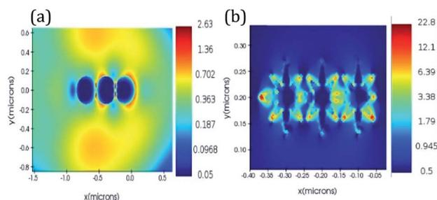
Fig. 1 FDTD simulations of electric field enhancement in (a) Au nanospheres (diameter = 100 nm) and (b) Au nano-urchins (diameter = 100 nm) at an excitation wavelength of 633 nm.
