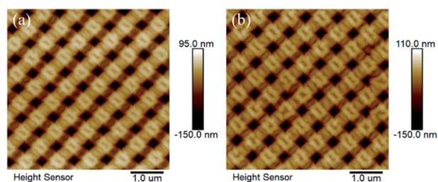
Fig. 3 AFM images of multiscale grid/wrinkle PDMS films with etching times of (a) 30 s and (b) 60 s.
