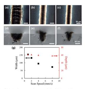
Fig. 3 Digital microscope images of the fabricated line structures. Surface of the structures fabricated with scan speed of (a) 1 mm s $^{-1}$ , (b) 4 mm s $^{-1}$ , and (c) 8 mm s $^{-1}$ , respectively. Cross sections of the structures fabricated with scan speed of (d) 1 mm s $^{-1}$ , (e) 4 mm s $^{-1}$ , and (f) 8 mm s $^{-1}$ , respectively. Structures were fabricated with a laser power of 150 mW. (g) Change in line width (black) and depth (red) with respect to scan speed.
