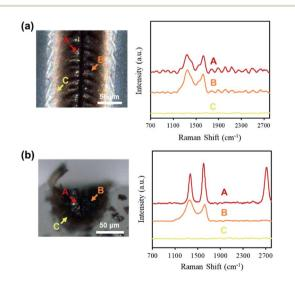
Fig. 5 Raman spectra taken for different areas of the (a) surface, and (b) cross section. Structures were fabricated with laser power of 150 mW and scan speed of 2 mm s<sup>-1</sup>. Arrows indicate the location of analysis, and color of arrow corresponds to the color of the resulting Raman spectrum.
