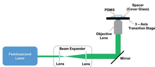
Fig. 1 Schematic illustration of the laser irradiation setup.
