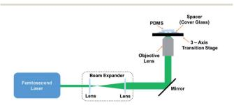
Fig. 1 Schematic illustration of the laser irradiation setup.
