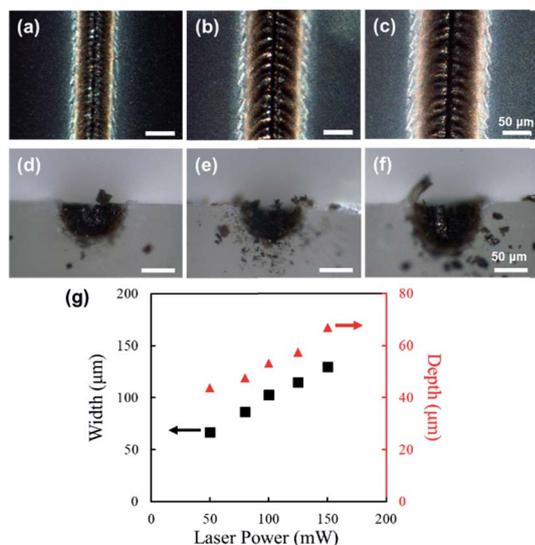
Fig. 2 Digital microscope images of the fabricated line structures. Surface of the structures fabricated with laser power of (a) 50 mW, (b) 100 mW, and (c) 150 mW, respectively. Cross sections of the structures fabricated with laser power of (d) 50 mW, (e) 100 mW, and (f) 150 mW, respectively. Structures were fabricated with a scan speed of  $2 \text{ mm s}^{-1}$ . (g) Change in line width (black) and depth (red) with respect to laser power.
