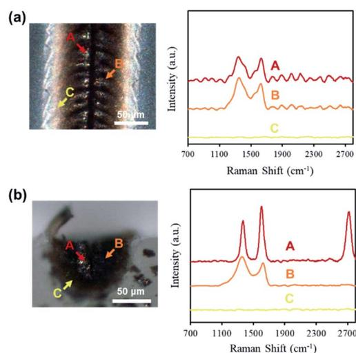
Fig. 5 Raman spectra taken for different areas of the (a) surface, and (b) cross section. Structures were fabricated with laser power of 150 mW and scan speed of  $2 \text{ mm s}^{-1}$ . Arrows indicate the location of analysis, and color of arrow corresponds to the color of the resulting Raman spectrum.
