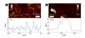
Fig. 3 AFM images and the corresponding height analysis of samples (a) without and (b) with 600  $\mu L$  of the methanol additive.
