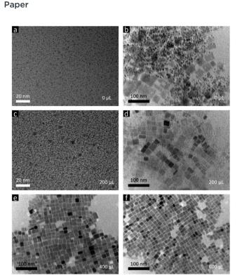
Fig. 2 TEM images of the final products from the LARP approach using different amounts of methanol: (a) and (b) 0  $\mu$ L, (c) and (d) 200  $\mu$ L, (e) 400  $\mu$ L, and (f) 600  $\mu$ L.
