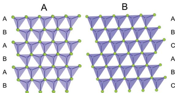
Fig. 2 Illustration of the stacking sequence in the wurtzite structure (A) and the zinc-blende structure (B). Cations are represented as purple dots, and anions are represented as green dots. The tetrahedrally coordinated Cd cations are shown to emphasize the layering of the structure.
