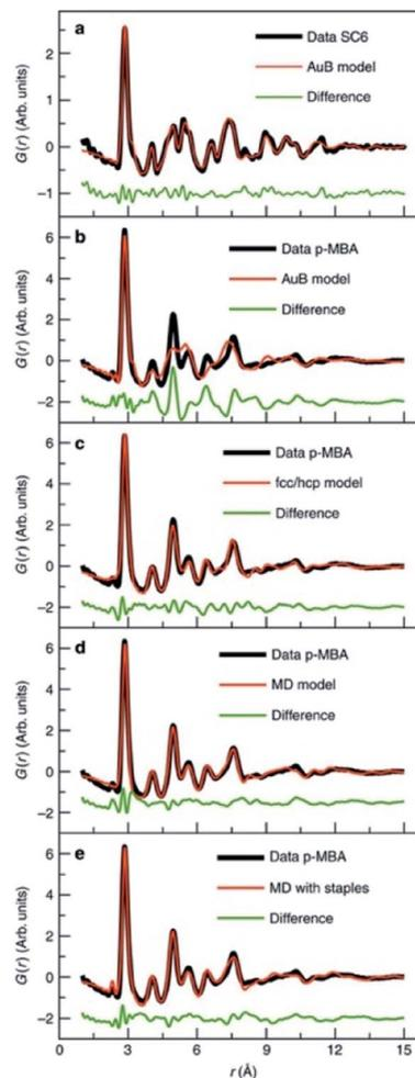
Fig. 10 Fits to experimental PDFs from Au<sub>144</sub>(SR)<sub>60</sub> samples. (a) Fit of an icosahedral structure model to data collected from Au<sub>144</sub>(SC)<sub>60</sub>. (b) Fit of an icosahedral structure model, (c) of an fcc/hcp model, (d) a 114 atom decahedral model and (e) a decahedral model with ‘staples’ to the PDF obtained from Au<sub>144</sub>(*p*-MBA)<sub>60</sub>. From Jensen *et al.*, *Nat. Commun.*, 2016, 7, 11859.<sup>140</sup>
