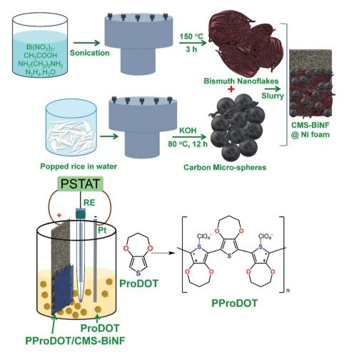
Scheme 1 Cartoon showing the preparation of the counter electrode for the QDSC.
