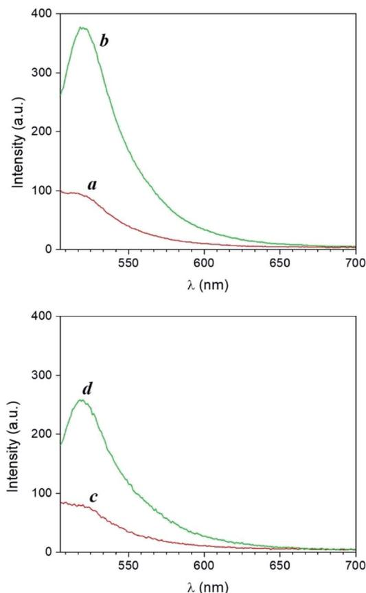
Fig. 5 Top: Emission spectra of a PVP (55 kDa, 20% w/v in MeOH) film containing **1** (500  $\mu$ M,  $\lambda_{\text{Ex}} = 490$  nm) and **3** (10 mM) before (a) and after (b) exposure at 254 nm for 40 min. Bottom: Emission spectra of a PVP (55 kDa, 20% w/v in MeOH) film containing **1** (500  $\mu$ M,  $\lambda_{\text{Ex}} = 490$  nm) and **4** (10 mM) before (c) and after (d) exposure at 365 nm for 40 min.
