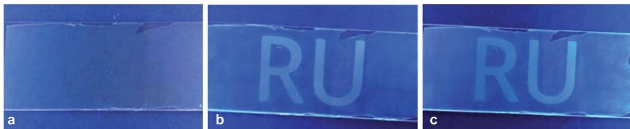
Fig. 6 Photographs of a thin PVP (55 kDa, 20% w/v in MeOH) film containing **1** (500  $\mu$ M) and **3** (10 mM) before (a), immediately (b) and 10 minutes (c) after exposure at 254 nm for 20 min through a RU-shaped 3D printed mask.
