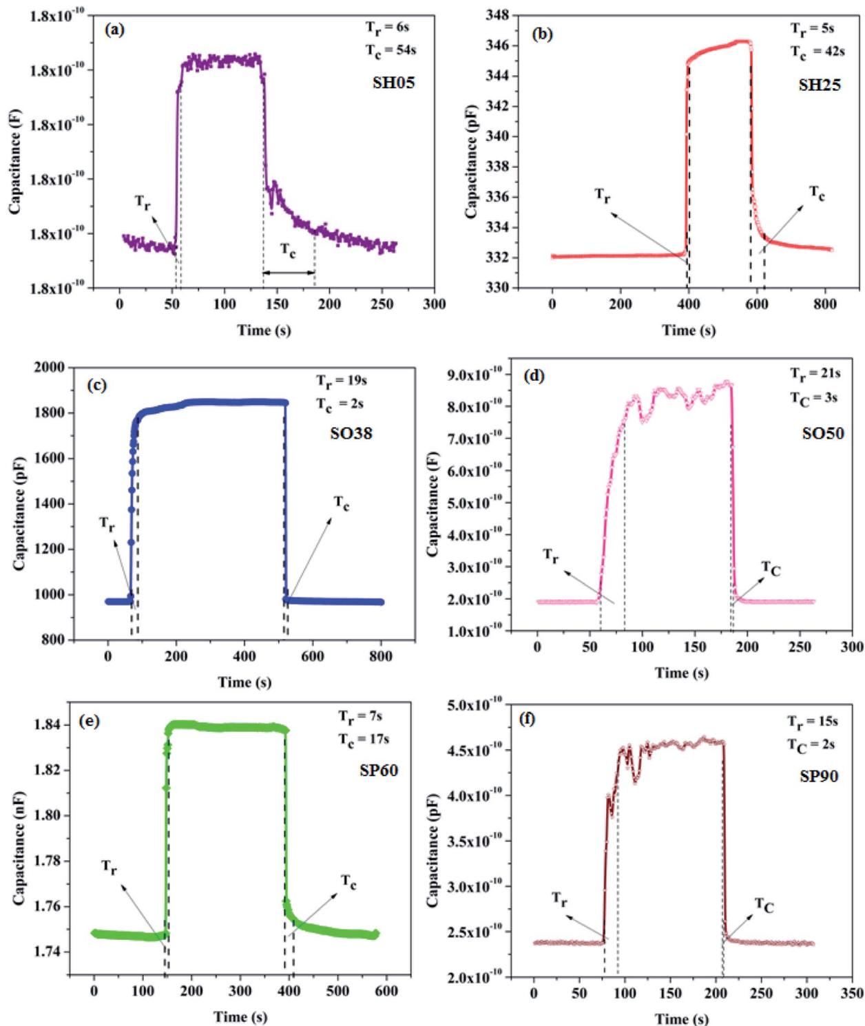
Fig. 11 Transient responses exhibiting the response and recovery times of the prepared sensors (a) SH05, (b) SH25, (c) SO38, (d) SO50, (e) SP60 and (f) SP90 at 50 RH%.
