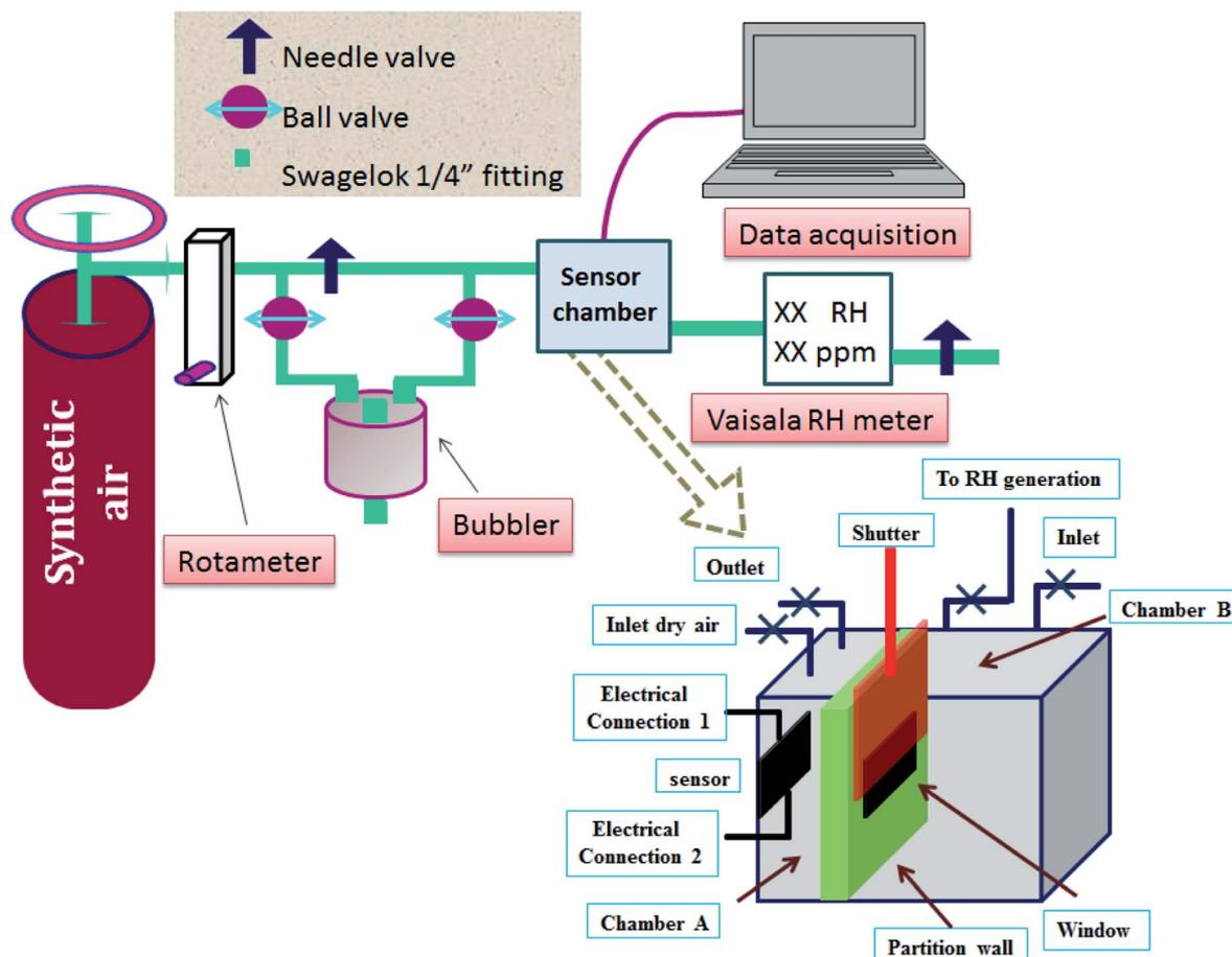
Fig. 3 Schematic diagram of the humidity sensing setup.
