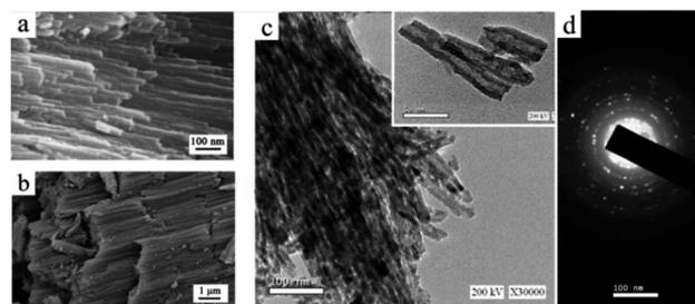
Fig. 3 (a) High resolution FESEM image of a TiO<sub>2</sub> single bundle confirming the aligned tubular arrays; (b) FESEM image showing TiO<sub>2</sub> bundles with smooth walls. (c) TEM image for the TiO<sub>2</sub> nanotube bundle after annealing; inset: TEM image of TiO<sub>2</sub> NTs before annealing, confirming the hollow structure. (d) Diffraction pattern of the TiO<sub>2</sub> NTs.
