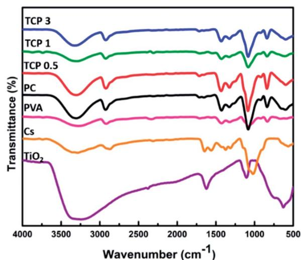
Fig. 8 FTIR spectra of TiO<sub>2</sub>, Cs, PVA, PC, and TCP nanofibrous materials.
