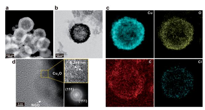
Fig. 3 (a) HAADF-STEM and (b) TEM image with (c) the corresponding elemental mapping images of NGO/Cu<sub>2</sub>O SPs. (d) High-resolution TEM image and the corresponding digital diffractograms of  $Cu_2O$ .
