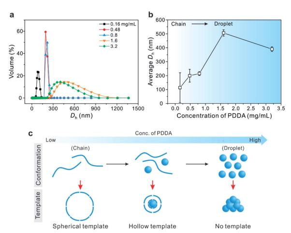
Fig. 2 (a) Volume distribution and (b) the corresponding average hydrodynamic diameter ( $D_h$ ) of PDDA by DLS upon increasing the PDDA concentration in the presence of 0.10 M Cu(OAc)<sub>2</sub>. (c) A schematic illustration of the conformational transition of the PDDA template from a chain to a droplet with increasing concentration of PDDA.
