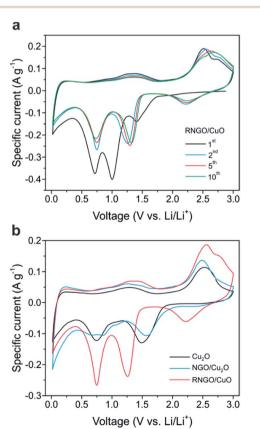
Fig. 5 CV curves of (a) RNGO/CuO SPs for various electrochemical cycles and (b) comparison of CV curves of Cu<sub>2</sub>O, NGO/Cu<sub>2</sub>O, and RNGO/CuO from the  $2^{nd}$  cycle at a scan rate of 0.10 mV s<sup>-1</sup> over the voltage range 0.02 to 3.0 V vs. Li/Li<sup>+</sup>.
