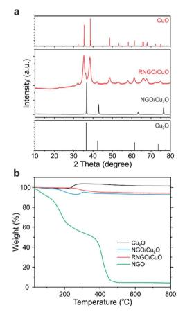
Fig. 4 (a) XRD patterns and (b) TGA of NGO/Cu<sub>2</sub>O and RNGO/CuO nanocomposites compared to bare  $\rm Cu_2O$  and NGO.
