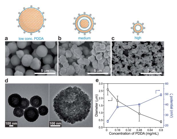
Fig. 1 Morphology transformation of Cu<sub>2</sub>O SPs assisted by the PDDA surfactant. SEM images of Cu<sub>2</sub>O SPs prepared at various PDDA concentrations: (a) 0.016, (b) 0.16, and (c) 0.80 mg mL<sup>-1</sup>, with a corresponding schematic illustration. (d) Representative TEM images of hollow Cu<sub>2</sub>O SPs from sample c when 0.80 mg mL<sup>-1</sup> PDDA was used. (e) Diameter and zeta potential of Cu<sub>2</sub>O SPs prepared with different concentrations of PDDA.
