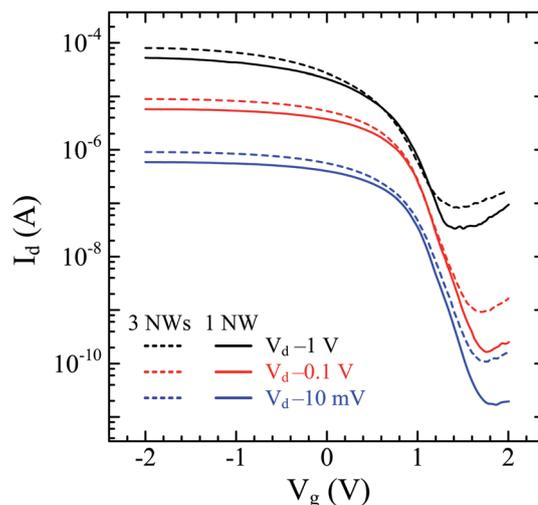
Fig. 5 Transfer characteristics ( $I_d$  versus  $V_g$  curve) of the devices consisting of a single nanowire (solid curves) and three nanowires (dashed curves) at a  $V_d$  of  $-0.01$  V,  $-0.1$  V and  $-1$  V. The gate voltage ( $V_g$ ) was swept from  $-2$  to  $2$  V. The channel length is  $1 \mu\text{m}$ .
