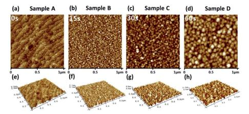
Fig. 3 AFM images of the four samples with different in situ NP growth times. (a-d) are the planar views, and (e-h) are the 3D views of the four samples, respectively.
