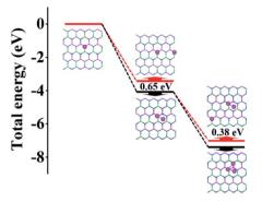
Fig. 2 The total energy of Al atoms adsorbed one by one on the Al<sub>0.5</sub>Ga<sub>0.5</sub>N surface.
