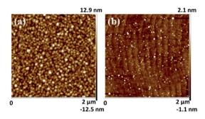
Fig. 5 The AFM surface morphology of in situ NP growth samples before (a) and after (b)  $\rm H_3PO_4$  etching.
