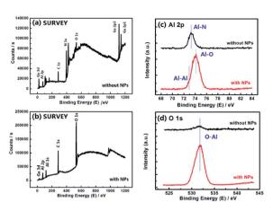
Fig. 4 (a and b) are XPS survey scan spectra of the samples with and without surface NPs. (c) is Al 2p core-level XPS spectra, and (d) is O 1s core-level XPS spectra of the samples with and without NPs.
