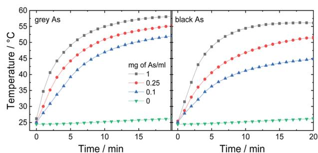
Fig. 7 Photothermic effect measured on three different As concentrations using an 880 nm ( $0.8 \text{ W cm}^{-2}$ ).
