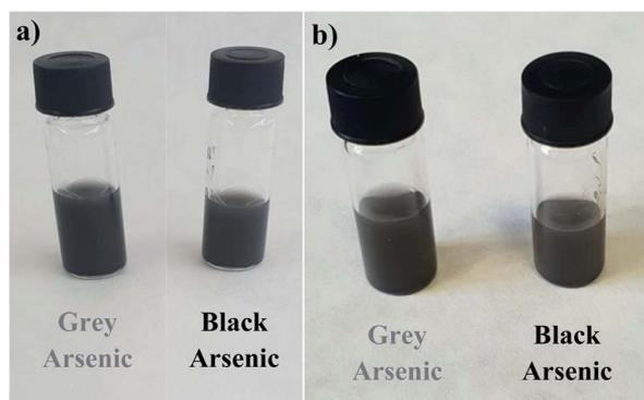
Fig. 2 Suspensions of exfoliated grey (left) and black (right) arsenic in acetonitrile (a) after 1 hour and (b) after 8 days.
