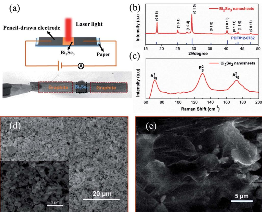
Fig. 2 (a) Schematic diagram of the experimental setup, inset: digital photograph of the real device. (b) XRD spectra of the  $\text{Bi}_2\text{Se}_3$  nanosheets. (c) Raman spectrum of  $\text{Bi}_2\text{Se}_3$  nanosheets. (d) Low-magnification SEM images of the liquid-exfoliated  $\text{Bi}_2\text{Se}_3$  nanosheets, inset: high-magnification SEM images of the liquid-exfoliated  $\text{Bi}_2\text{Se}_3$  nanosheets. (e) SEM images of pencil-drawn electrodes.
