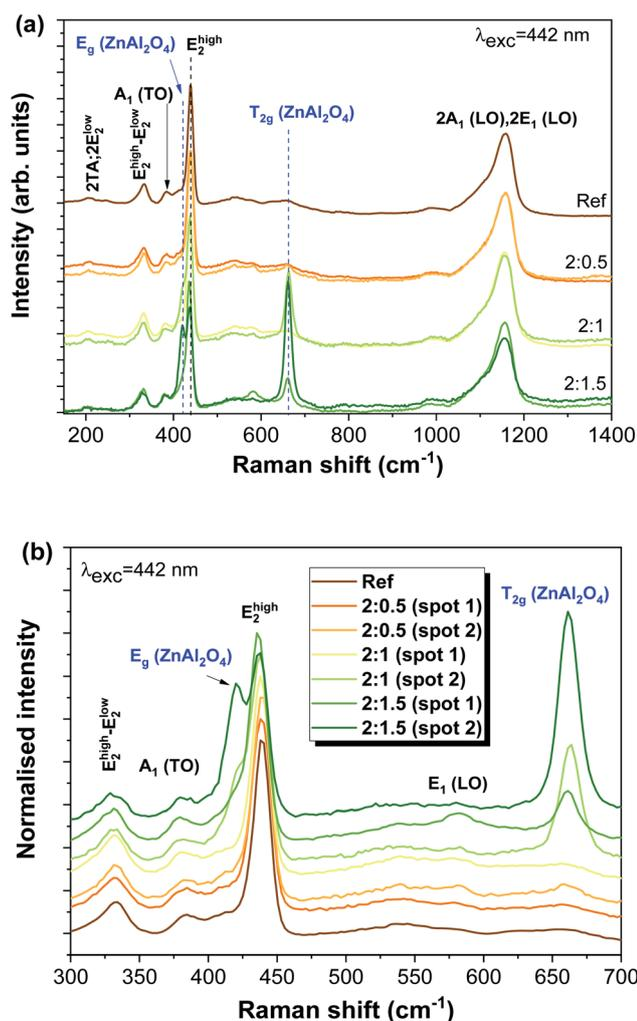
Fig. 3 (a) RT Raman spectra of the Al-doped ZnAl<sub>2</sub>O<sub>4</sub>/ZnO tetrapodal networks with increasing ZnO : Al ratios, obtained with 442 nm laser line excitation. The spectra were shifted vertically for clarity. (b) Enlarged view of the  $E_2$  (high) mode spectral region.
