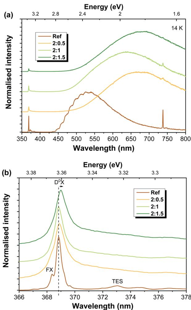
Fig. 4 Low temperature PL spectra obtained under 325 nm laser excitation for Al-doped  $\text{ZnAl}_2\text{O}_4/\text{ZnO}$  structures (a) in the UV-Vis range and (b) with high resolution in the NBE region.
