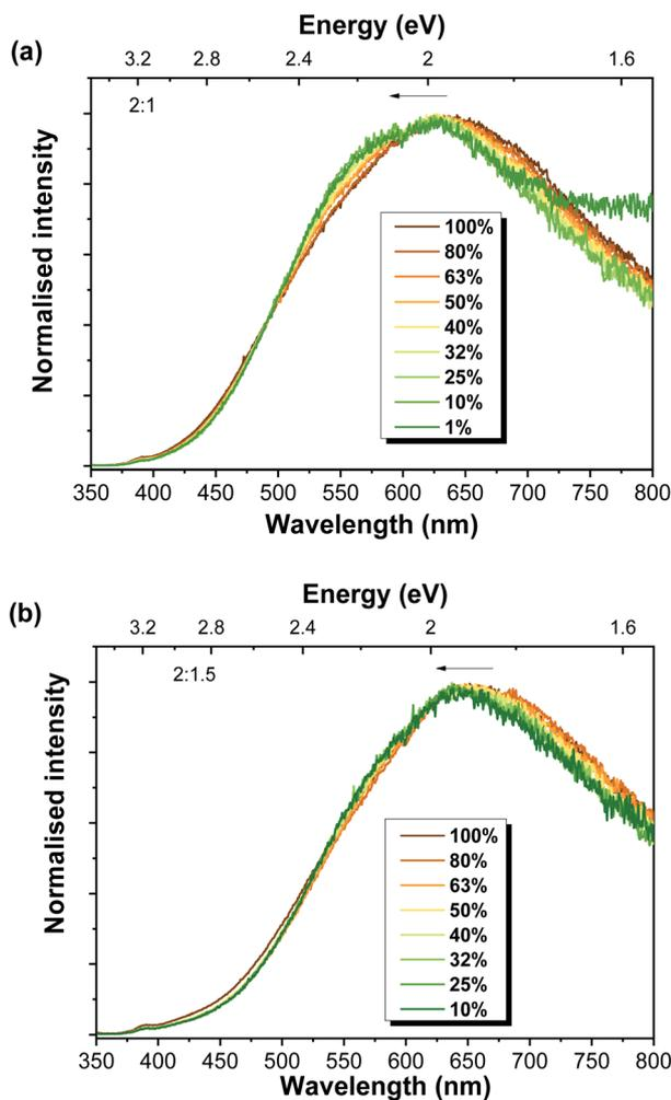
Fig. 6 RT power-dependent PL spectra for the Al-doped ZnO/ZnAl<sub>2</sub>O<sub>4</sub> samples with ZnO : Al ratios of (a) 2 : 1 and (b) 2 : 1.5.
