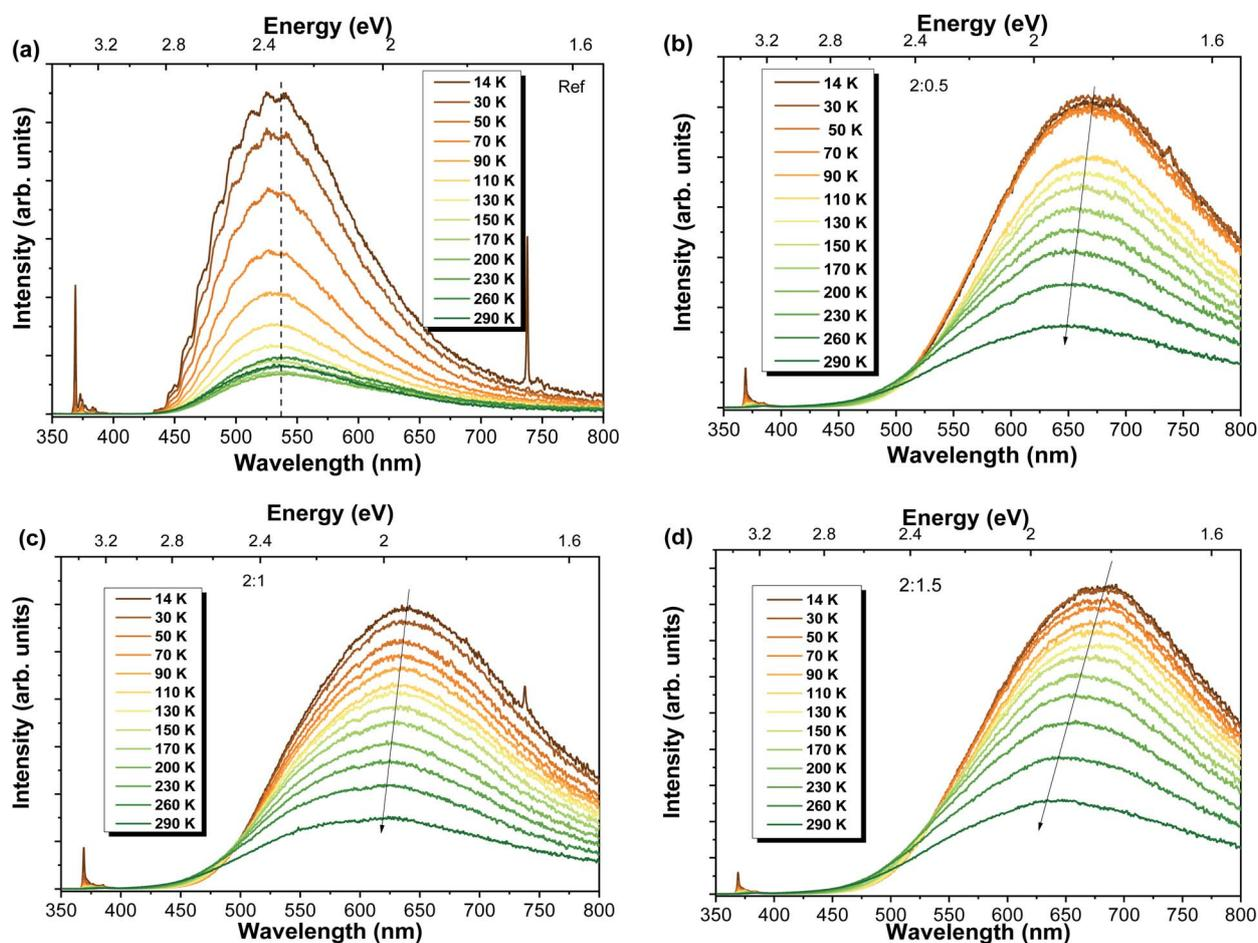
Fig. 5 Temperature-dependent PL spectra obtained under 325 nm laser excitation for the Al-doped ZnO/ZnAl<sub>2</sub>O<sub>4</sub> samples: (a) reference sample and samples with different ZnO : Al ratios (b) 2 : 0.5, (c) 2 : 1 and (d) 2 : 1.5.
