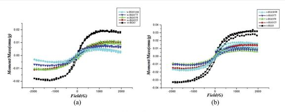
Fig. 12 Magnetization versus field measurements for (a) w-RGO and (b) s-RGO at different  $\gamma$ -irradiation doses. Reproduced with permission from ref. 70, copyright 2019, Elsevier.
