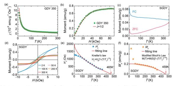
Fig. 9 (a) Typical susceptibility—temperature ( $\chi$ –T) curve for GDY-350. (b) M–H curve for GDY-350 measured at temperature 2 K. (c) Magnetization *versus* temperature (M–T) curves for SGDY. (d) Magnetization *versus* field (M–H) curves for SGDY. (e) Coercivity variation with temperature for SGDY. (f) M–T curve fitted by the modified Bloch's law. Reproduced with permission from ref. 45, copyright 2019, American Chemical Society.
