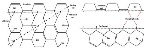
Fig. 13 (a) A pictorial representation of unzipping of graphene oxide via (b) zig-zag and/or armchair cutting
