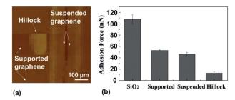
Fig. 9 (a) Adhesion force map covering the SiO<sub>2</sub> substrate, the supported graphene, the suspended graphene, and the hillock-like structure on the SiO<sub>2</sub>/graphene surface. (b) Statistics of the adhesion force on the above four surfaces
