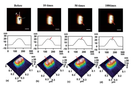
Fig. 4 Indentation tests with different numbers of indenting cycles on the hillock-like structure surface. (a) A hillock-like structure on the supported monolayer graphene surface before the indentation tests; (b), (c), and (d) show the topography variation of the hillock-like structure with the number of indentation cycles of 10, 50, and 100 times, respectively. The applied normal load  $F_n$  during such tests was 1  $\mu$ N. The scale bars in the AFM images were 50 nm.
