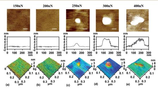
Fig. 5 Effect of normal load on the friction-induced hillock structure on the bare  $SiO_2$  surface. The sliding tests are performed on five regions with an area of 100 nm  $\times$  100 nm under the normal loads of 150 nN, 200 nN, 250 nN, 300 nN and 400 nN, respectively. The scale bars in this figure are 60 nm.
