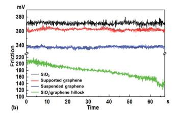
Fig. 7 Measurement of friction force on the SiO<sub>2</sub> substrate, supported graphene, suspended graphene and the hillock-like structure on the SiO<sub>2</sub>/graphene surface under the normal loads of 5 nN (a) and 10 nN
