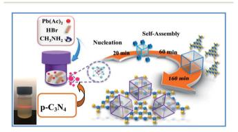
Fig. 1 Schematic illustration of the formation and morphological evolution process of  $MAPbBr_3/p-g-C_3N_4$  composites using a p-g-C<sub>3</sub>N<sub>4</sub> sol solution through a solvothermal method.
