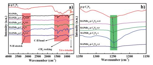
Fig. 3 (a and b) Full and partial regional FTIR spectra of products prepared with different contents of p-g- $C_3N_4$  confirming that the C-N-Br chemical bonding interaction is present in MAPbBr<sub>3</sub>/p-g- $C_3N_4$ .
