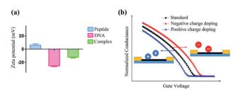
Fig. 6 (a) Zeta potential values of the CW peptide, DNA, and their complex. The electrostatic adsorption of the peptide and DNA occurred because of their opposite ZP and the formed complex had the same ZP as DNA, which hindered the continuous adsorption with DNA. (b) Illustration of the current change sensitive to charge doping. The negative charge doping induced a right shift of the characteristic curve, resulting in an enhanced current and vice versa:
