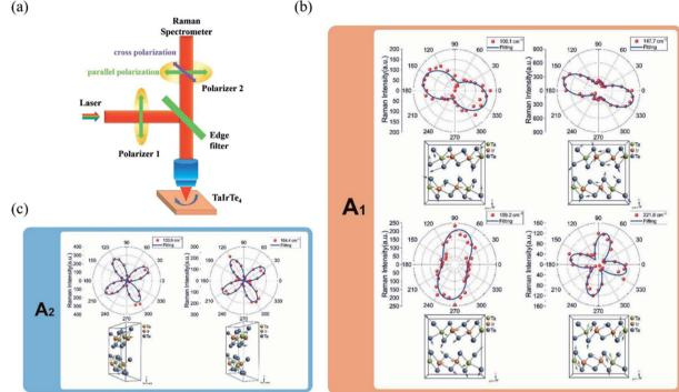
Fig. 8 (a) Schematic of the angle-resolved polarized Raman spectroscopy of TalrTe $_4$  samples. Raman intensities of (b)  $A_1$  and (c)  $A_2$  modes as a function of the sample rotation angle and the corresponding phonon modes in the atomic view. The scattered dots are the experimental data and the solid lines are the fitting curves. Reproduced from ref. 49 with permission from Wiley-VCH.
