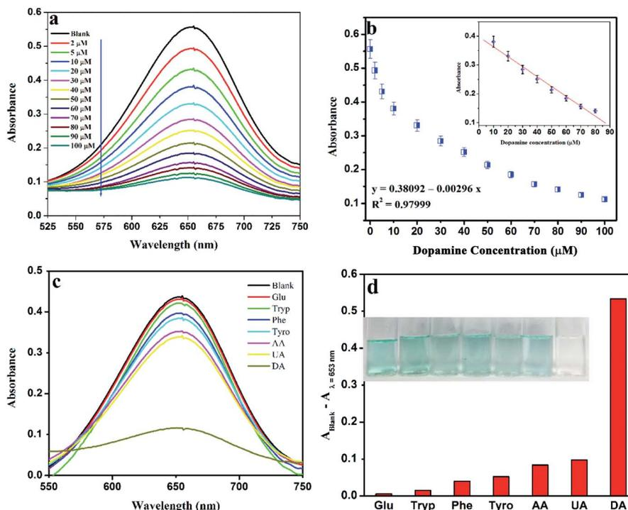
Fig. 11 (a) UV-vis spectra of TMB oxidation in the presence of a variable amount of DA (b) linear calibration plot for DA (c) UV-vis spectra of TMB oxidation in the presence of 100  $\mu M$  various interfering species, and (d) comparison with other substrates.
