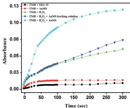
Fig. 6 Time-dependent absorption curve for the TMB–H<sub>2</sub>O<sub>2</sub> system using AuMS at 653 nm under different conditions.
