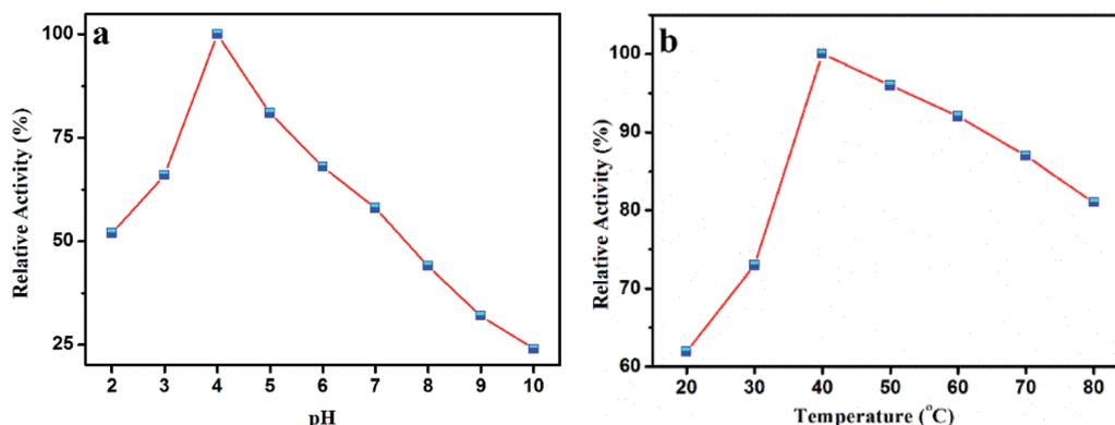
Fig. 7 (a) Effects of pH and (b) temperature on the catalytic oxidation of TMB in the presence of AuMS and H<sub>2</sub>O<sub>2</sub>.
