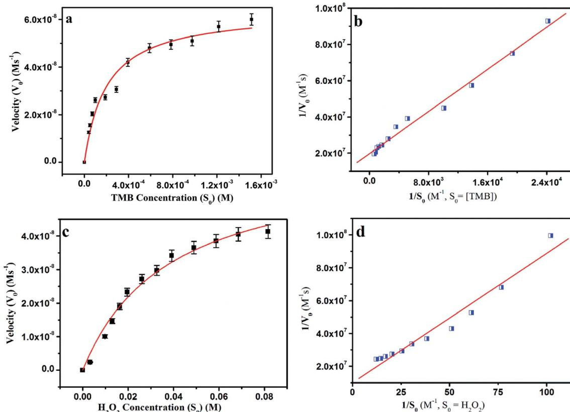
Fig. 9 Steady-state kinetic analyses using the Michaelis–Menten model and Lineweaver–Burk model for AuMS by (a and b) varying the concentration of TMB with a fixed amount of  $\text{H}_2\text{O}_2$  and (c and d) varying the concentration of  $\text{H}_2\text{O}_2$  with a fixed amount of TMB.
