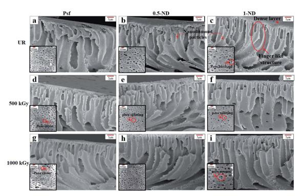
Fig. 4 SEM images of the cross-section of the membrane with and without NDs: (a–c) unirradiated (UR) membranes, (a) Psf, (b) 0.5-ND, and (c) 1-ND; (d–f) exposure to a 500 kGy radiation dose, (d) Psf-500, (e) 0.5-ND-500, and (f) 1-ND-500; (g–i) exposure to a 1000 kGy radiation dose, (g) Psf-1000, (h) 0.5-ND, and (i) 1-ND-1000. Inset in the images shows the pores in the respective membranes.
