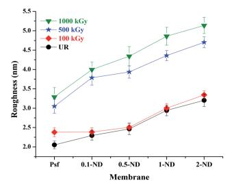
Fig. 5 Variations of RMS roughness of membranes at different loadings of NDs and radiation dose.
