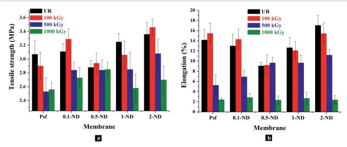
Fig. 12 Mechanical properties of membranes with the loading of NDs in the membrane matrix and gamma radiation dose: (a) variations in the tensile strength with loading of NDs into the membrane matrix and radiation dose; (b) changes in the percentage elongation at break of the membranes at maximum force with the loading of NDs and the radiation dose.
