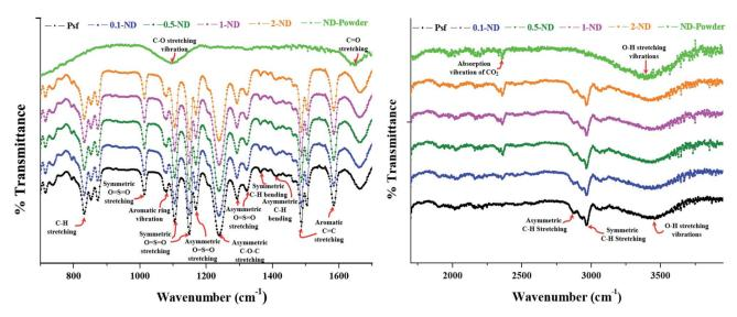
Fig. 7 ATR-FTIR spectrum of the unirradiated control Psf and Psf-ND composite membranes.
