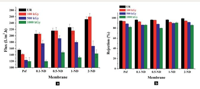
Fig. 13 Performance of the control Psf and Psf–ND composite membranes with loading of NDs and radiation dose: (a) permeability of membranes in terms of the flux of water through membranes (LMH), (b) rejection of polyethylene oxide (PEO, molecular weight 100 KDa) by the membranes.
