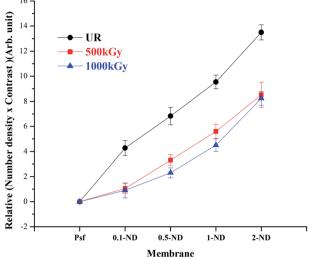
Fig. 11 Variation of relative "number density x contrast" of the membrane matrix obtained from SAXS with the loading of NDs at different radiation doses
