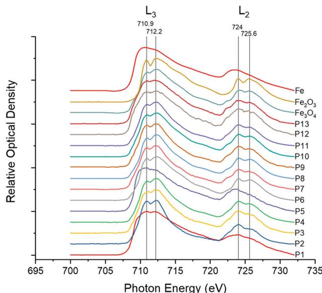
Fig. 2 XANES spectra of iron, iron(III) oxide ( $\text{Fe}_2\text{O}_3$ ) and iron(II,III) oxide ( $\text{Fe}_3\text{O}_4$ ) standards, with spectra of individual particles. Standard spectra represent averages over a single field of view. Sample UFPM spectra represent a single particle per spectrum. Peak photon intensities are shown for  $\text{Fe}_2\text{O}_3$  and  $\text{Fe}_3\text{O}_4$ .
