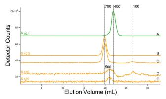
Fig. 10 Phosphorus (green, (A)) and sulfur (yellow, (B)-(E)) -detected chromatograms of cytosol FTSs. (A) From WT cells grown with 40  $\mu$ M Fe and 10  $\mu$ M Cu; isolated using buffer (C). (B) 10 mM MES buffer. (C) Same as in (A). (D) WT cells grown as in (A) but cytosol was isolated using 20 mM ammonium acetate. (E) Reduced glutathione (250 µM). A single treated column was used
