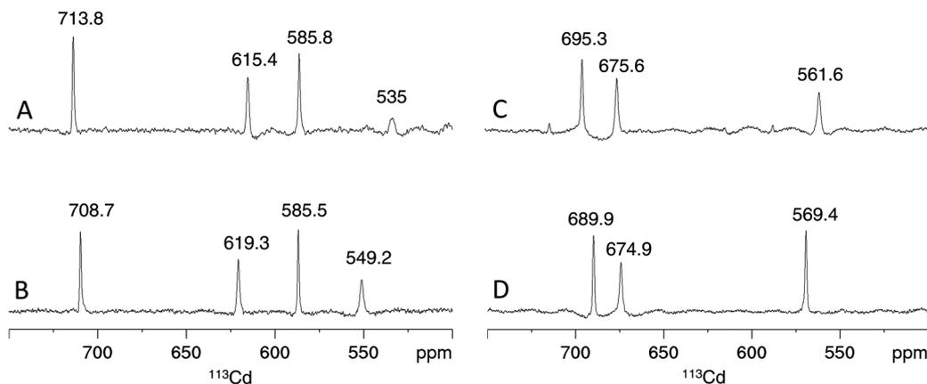
Fig. 5 Cadmium coordination environment in PflQ2 MT and the S29C mutant. Proton-decoupled 1D  $^{113}\text{Cd}$  spectra at 320 K of the  $\text{Cd}_4$  (A and B) and  $\text{Cd}_3$  (C and D) species of PflQ2 MT (A and C) and S29C-PflQ2 MT (B and D). Peak integrals are listed in Table S2 (ESI $^\dagger$ ).
