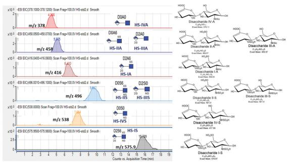
Fig. 4 Extracted ion chromatograms (EICs) for heparan sulfate (HS) disaccharide standards using GlycanPac AXH-1 (ThermoScientific) column mounted on an Agilent 1200 LC attached to an Agilent 6520 Q-TOF. ♦; ∆-uronic acid, ■; N-acetyl glucosamine.
