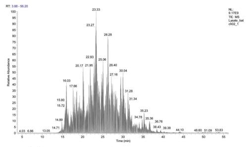
Fig. 5 Total ion chromatogram (TIC) for mouse brain tissue lysate after serial in-solution digestion protocol.
