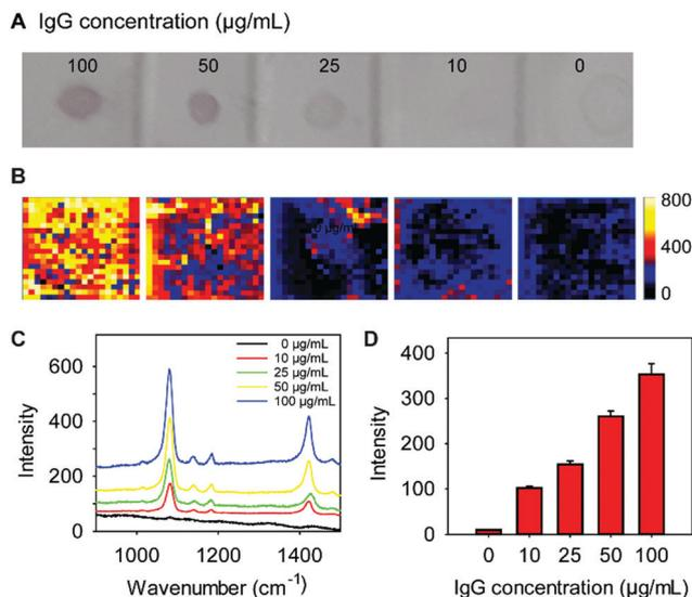
**Fig. 4** Sensitivity study: 1  $\mu\text{L}$  of different concentrations of IgG solutions were immobilized on a PVDF membrane and then incubated with WGA-SERS nanotags (A). The SERS image (Raman intensity) of each spot is shown in (B) with the average SERS spectra shown in (C). Relationship between SERS intensity and the concentration of IgG (D), where the average of 400 intensity measurements is presented.
