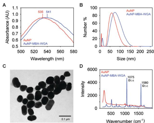
**Fig. 2** Characterization of lectin-SERS nanotags. (A) UV-Vis absorption spectra of AuNPs and lectin-SERS nanotags, where the absorbance maxima are indicated; (B) size distribution of AuNPs and lectin-SERS nanotags measured by dynamic light scattering; (C) TEM image of lectin-SERS nanotags, and (D) Raman spectra of AuNPs before and after functionalisation, where the peaks assigned to MBA vibrational modes are indicated.
