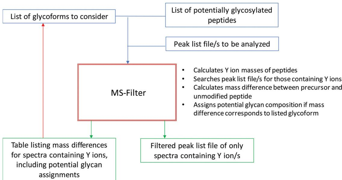
**Fig. 1** Flowchart of Y ion filtering process using MS-Filter. The input is peak list file/s and a list of candidate peptides. The user specifies parameters including how many Y ions need to be matched and at what mass tolerance, and what glycoforms to consider. The software outputs a new peak list file containing only those spectra that pass the filtering criteria, and also a table listing these spectra, the observed mass modification and potential glycan explanations for the masses.
