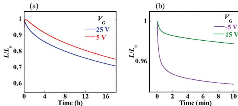
Fig. 5 (a) The operational lifetime of the red QD-HLET tested at different  $V_{GS}$  and a constant current density of  $71 \text{ mA cm}^{-2}$ . (b) The luminance as a function of time for the red QD-HLET with a loop test between  $-5 \text{ V}$  and  $15 \text{ V}$  of  $V_{GS}$  at a constant current density of  $71 \text{ mA cm}^{-2}$ .
