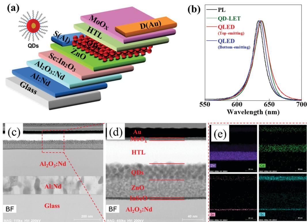
Fig. 2 (a) Device structure of the QD-HLET. (b) PL spectrum of the red QD film and normal EL spectra of the QD-HLET, bottom-emitting QLED and equivalent top-emitting QLED. (c and d) STEM images with different magnifications of the QD-HLET. (e) EDS mapping image of the QD-HLET.
