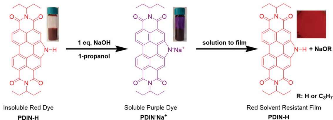
Fig. 1 Chemical structure of PDIN-H. Treatment of a 10 mg mL -1 slurry of PDIN-H in 1-propanol with 1 molar equivalent of NaOH produces a purple ionic solution. Spin-coating this solution onto a PET substrate yields a red colored organic film owing to the spontaneous protonation of the PDIN - anion. This process mimics that of classic acid dyeing of textiles.
