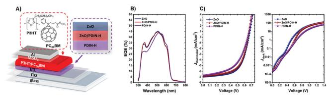
Fig. 9 (A) OPV device architecture. (B) EQE spectra. (C) Current density-voltage characteristics under 1-sun illumination (left) and in the dark (right). PDIN-H layer processed from PDIN-H solutions in 1-propanol with 1 molar equivalent of NaOH added.
