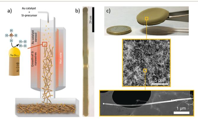
Fig. 1 Continuous synthesis of macroscopic networks of SiNWs by floating catalyst chemical vapour deposition. (a) Schematic of the synthesis process based on catalytic decomposition of SiH<sub>4</sub> in the presence of an aerosol of Au particles. (b) Photograph of continous SiNW tape on the metre scale. (c) Free-standing SiNW material and electron micrographs of the porous ensemble of long SiNWs.
